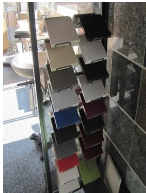
Photo 1: Display unit showing different shades and finishes of artificial stone with a high silica content. (Source: photo by Vincent Bonneterre)
