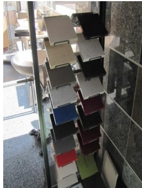
Photo 1: Display unit showing different shades and finishes of artificial stone with a high silica content. (Source: photo by Vincent Bonneterre)
